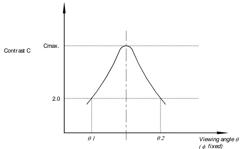
Note : Optimum vision with the naked eye and viewing angle  $\theta$  at  $C_{max}$  above are not always the same.
