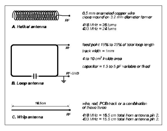
figure 6: Antenna configurations
