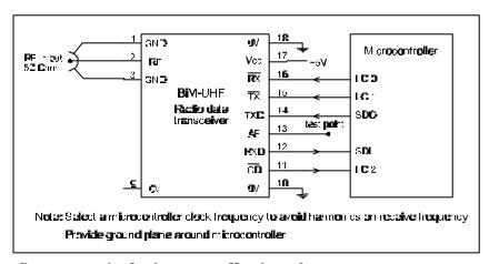
figure 7: typical microcontroller interface
