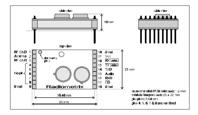
figure 2: mechanical dimensions
