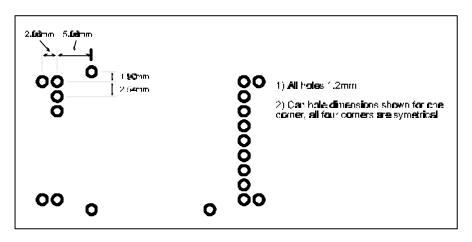
figure 12: hole pattern BiM-UHF + BiM-can
